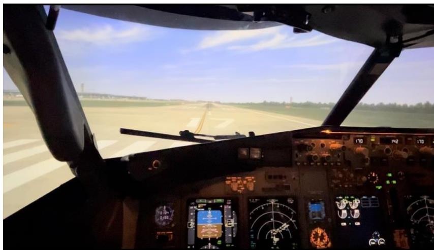
Figure 1. Flight deck of B737-800 FFS.
